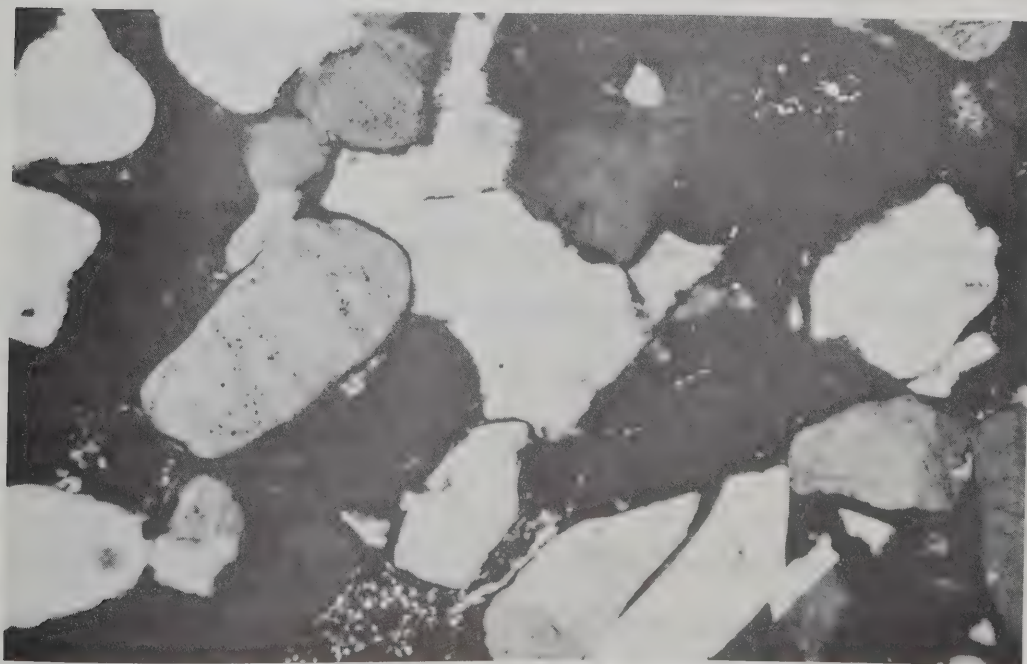
PLATE 7.7b A cemented orthoquartzite. The grains show little diagenetic alteration, but are cemented together. X130.
